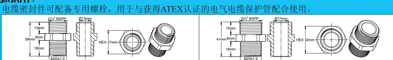
**气体类别:** Ex II 2G Ex eb db IIC T5 Gb; **粉尘分类:** Ex II 2D Ex tb IIIC T95°C Db
